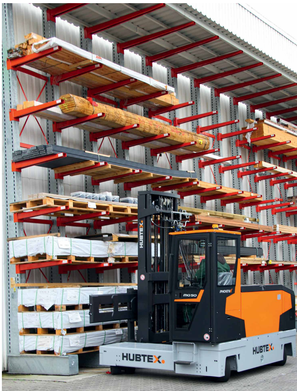
Above: Electric sideloaders provide flexible timber handling both indoors and outdoors.
