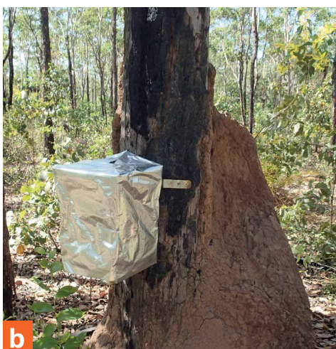
Figure 5: Exposure of wafers against Coptotermes acinaciformis : a) wafer/baitwood assembly in exposure container, b) exposure container installed in the field, c) wafers after take-down of the field trial.
