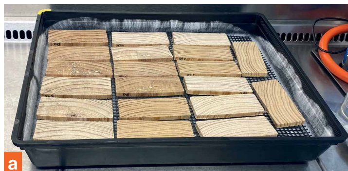
Figure 4. Wafers exposed to decay fungi in the laboratory: a) set-up, b) after 12 weeks' exposure.
