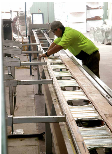
Above: Australian fabrication, whether cassette manufacture at Tilling’s Kilsyth plant shown above or standard frame and truss operators, is adaptable and accomplished. But it can’t move into multi-residential work without architects and engineers
