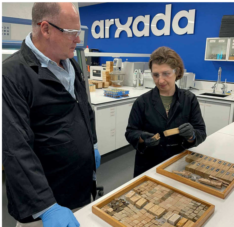
Above: Expert staff at Arxada's Technical Centre examined 720 timber billets exposed to rot and termites.
