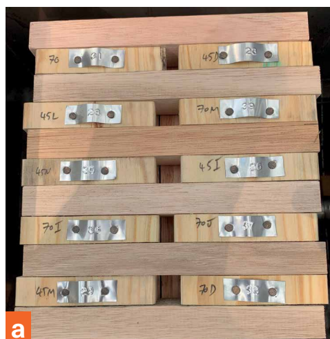
Figure 5: Exposure of wafers against Coptotermes acinaciformis : a) wafer/baitwood assembly in exposure container, b) exposure container installed in the field, c) wafers after take-down of the field trial.
