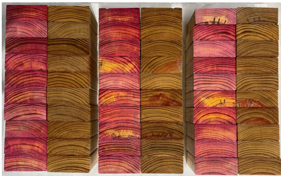
Figure 3: Example of spot tested billets with a range of preservative uptakes and gradients.
