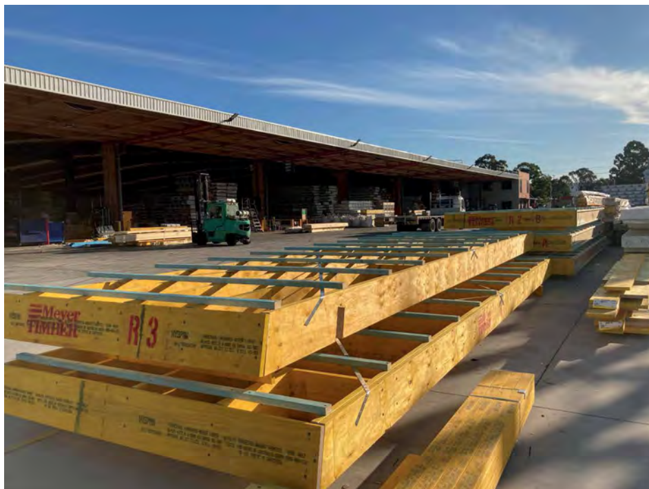
Above and opposite: Roof cassettes are finished to order off site, then craned directly into place on site.
