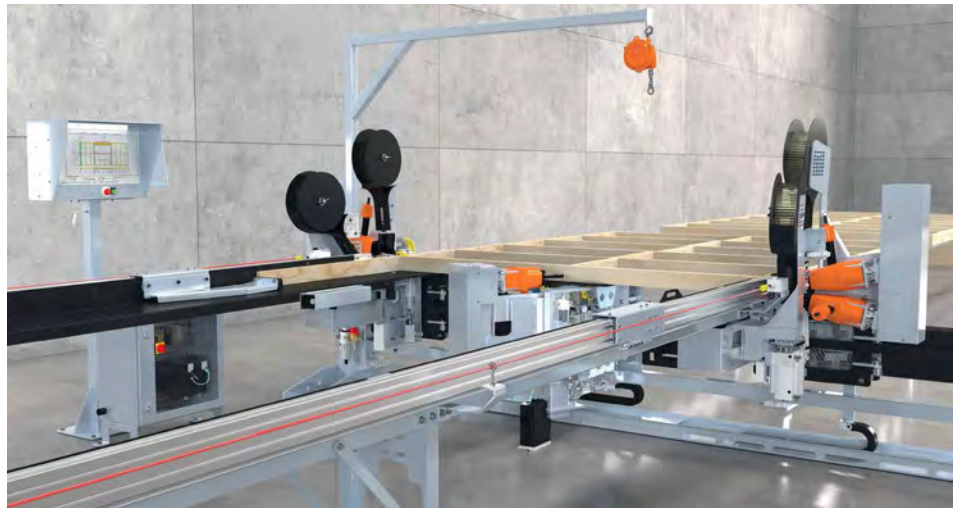
Above: Multinail's new Auto Framer speeds wall frame production and lowers the strain on labour.
