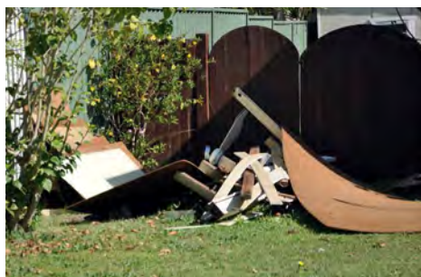
Above: Fibro sheeting and boards found under eaves and as linings are places you might expect to find asbestos, but it can also be in the adhesives and seals.
