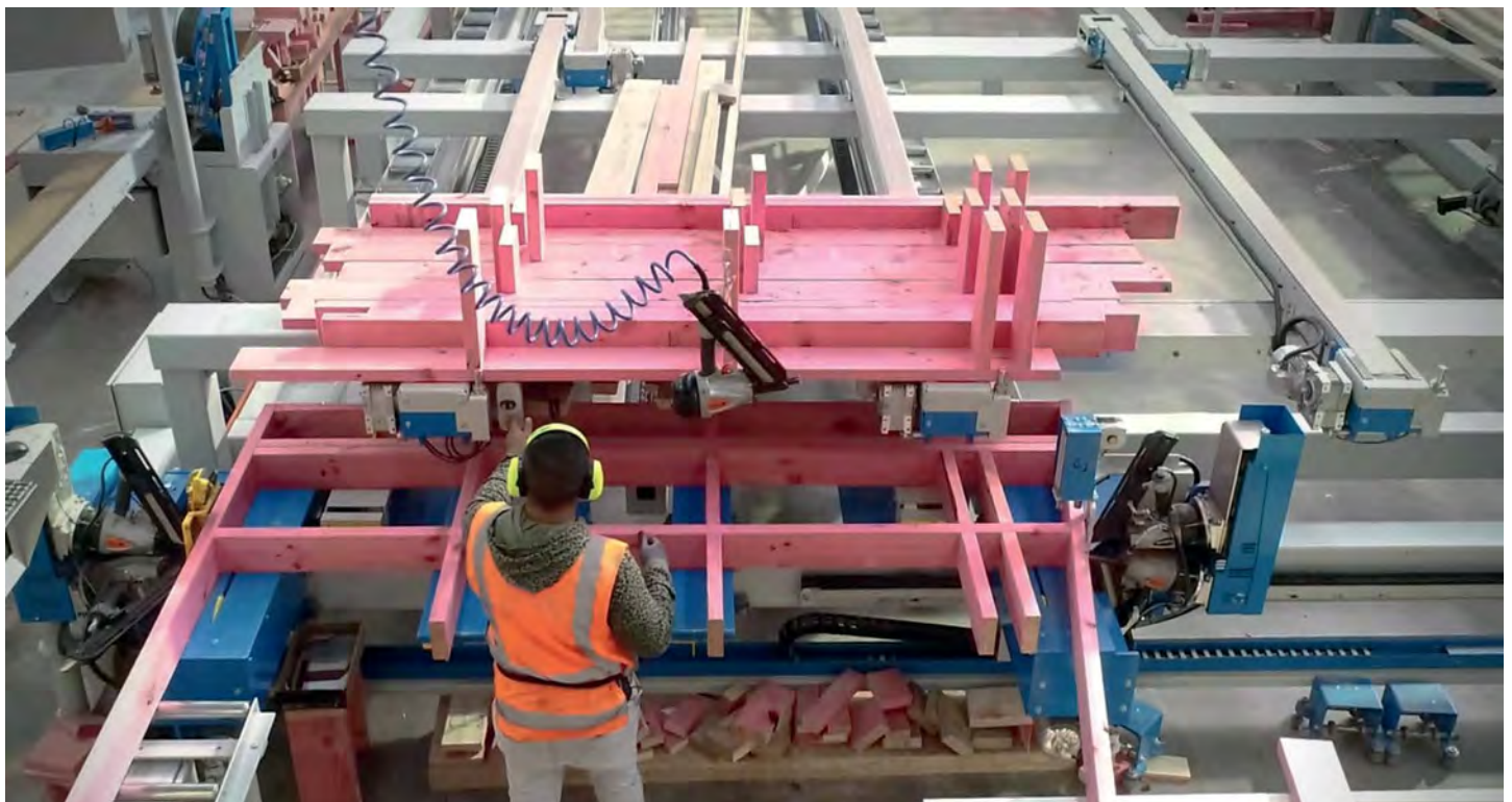
Above: The new Raked Wall Extruder simplifies frame production with the fast and automatic assembly of both raked and standard wall frames.
