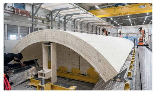
Above: The LVL towers are fabricated in sections, allowing for easier and cheaper transport to site.
