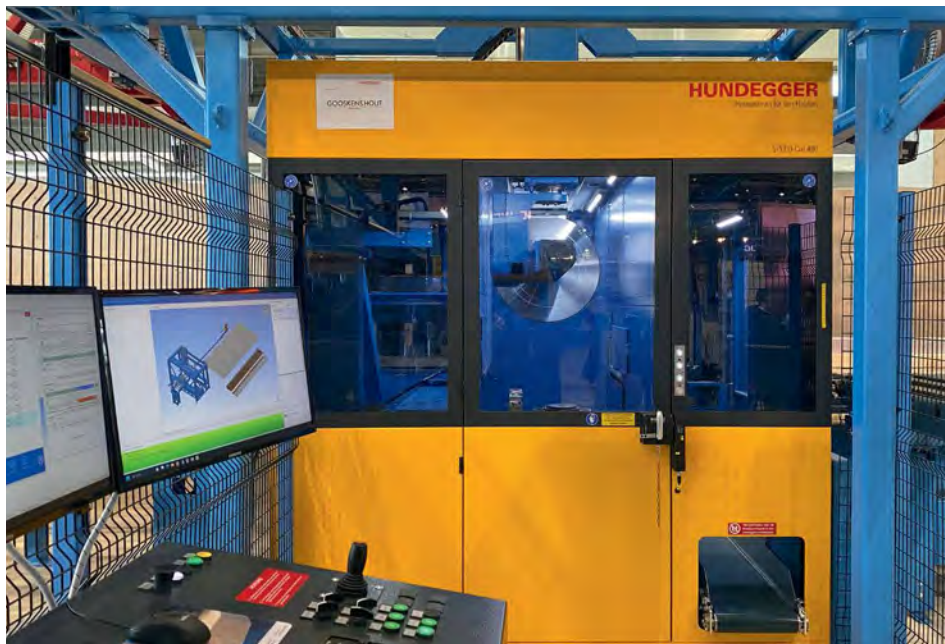
Above: The incredibly versatile Hundegger ROBOT-compact 650 (left) and the SPEED-Cut 480 – ideal for processing I-joist, glulam, LVL and solid timber.
