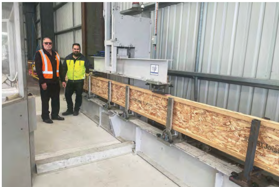
Above: Craig Kay (left) and Yuri Huerta testing an I-joist at Tilling's Melbourne manufacturing facility.
