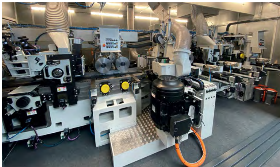
Above: Weinig's new Hydromat 4400 attracted a lot of attention with speeds over 400m/minute.
