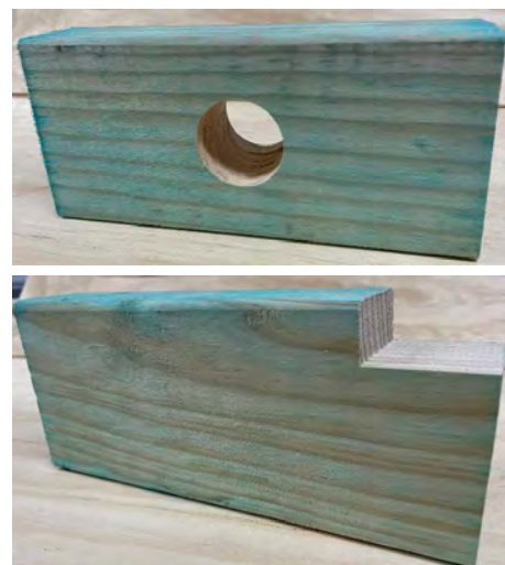
Above: Fig 2. Example of framing samples with a) notch, and b) drilled hole, exposed to Coptotermes acinaciformis in field trials.
