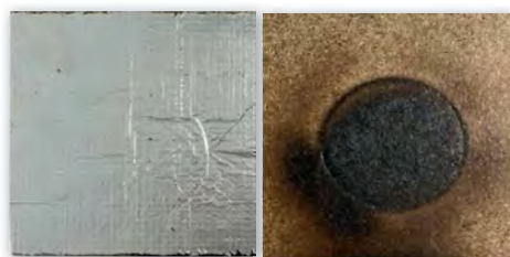
Above: The same flame test on R-Flor, left and Structaflor, showing R-Flor's higher resistance.
