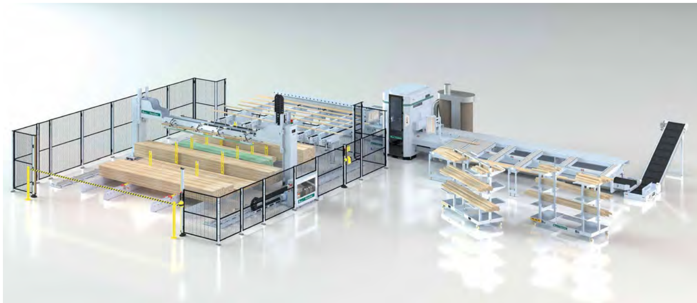
Above: Multinail's new PieceGiver system automates the infeed to the company's popular PieceMaker saw, dramatically speeding cutting time.
