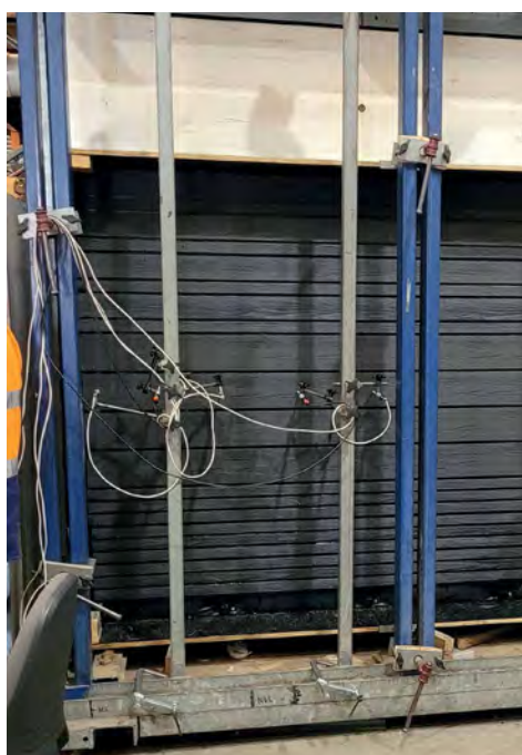
Above: Testing the VistaClad system against Australian Standards took three weeks, including building walls and then testing to destruction – in the end the screws holding the Clip Strips to the studs were what failed.
